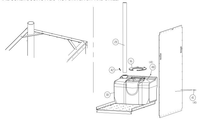
9. TIGHTEN ALL REMAINING BOLTS AND NUTS TO THE TOP ANGLES AT THIS TIME WITH 7/16" SOCKET AND WRENCH.
