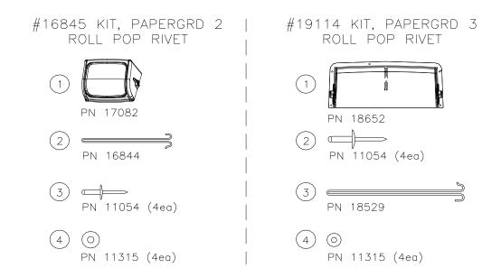
LOCATE PAPERGUARD ON LEFT PANEL AS SHOWN. MARK THE (4) HOLES ON THE INSIDE OF THE PAPERGUARD WITH MARKER. DRILL OUT THE (4) MARKED SPOTS ON PANEL WITH A 1/4" DRILL BIT. FASTEN PAPERGUARD HOOD WITH THE #11054 RIVETS FROM THE OUTSIDE AND #11315 WASHERS ON THE INSIDE OF TOILET. SLIDE #16844 SPINDLE IN PAPERGUARD.
