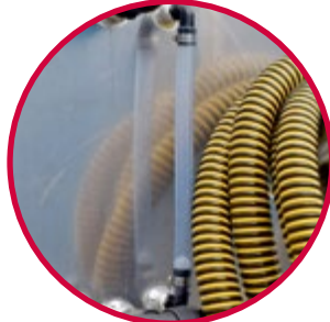
Easy-to-gauge sight tube for fresh water level.
